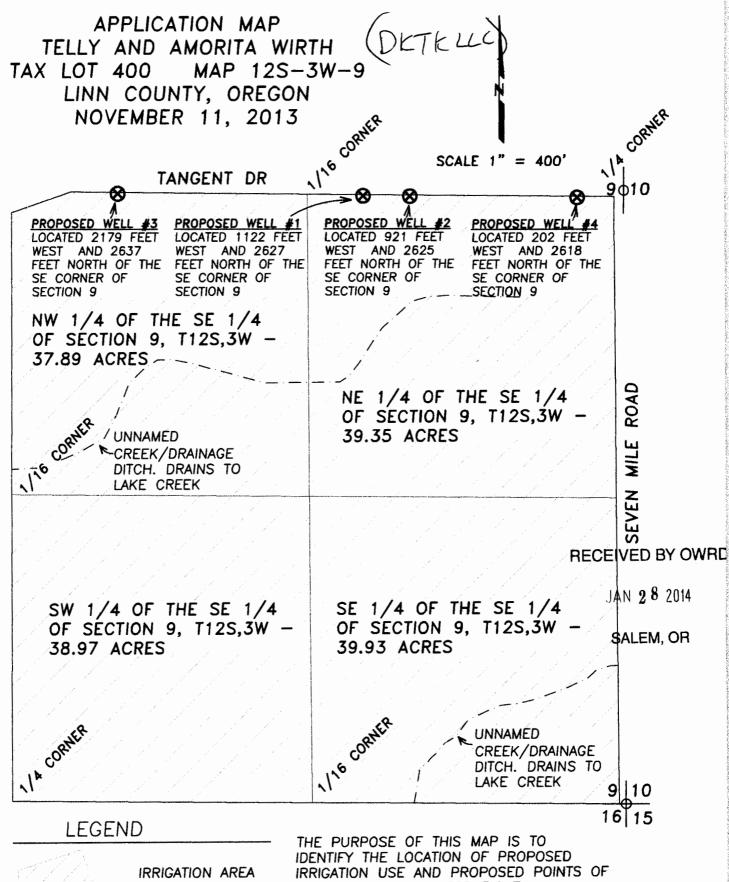
DIVERSION FOR A WATER RIGHT APPLICATIOIN. THIS IS NOT A BOUNDARY SURVEY.
