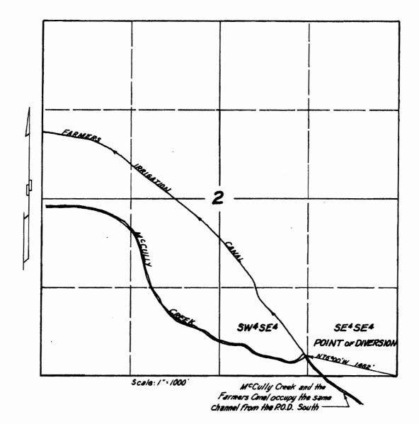
POINT OF DIVERSION: Taken at the point where the flood water of MCCully Creek are diverted into the Farmers Canal and which bears N76°00'W a distance of 1462 feet from the SE corner of Sec. 2, T25, R45 E.W.M.
