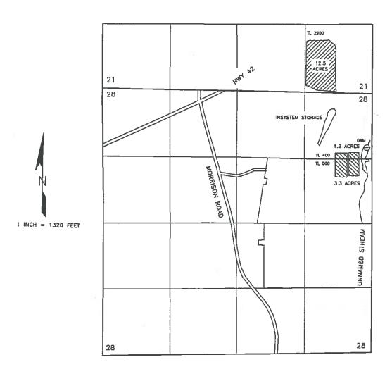
THE POINT OF DIVERSION IS LOCATED 1,40 FEET SOUTH AND 112 FEET WEST FROM THE NORTHEAST CORNER OF SECTION 28, AND WITHIN THE NEWNEW OF SECTION 28, TOWNSHIP 28 SOUTH, RANGE 14 WEST, W.M., COOS COUNTY.
