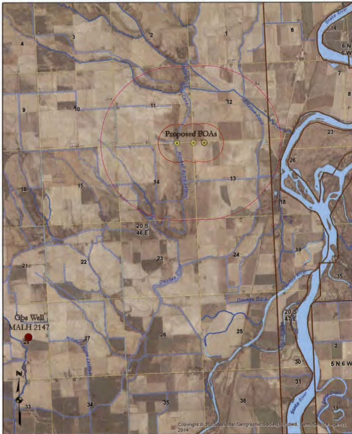
Figure 3: Proposed wells are greater than one mile from any natural surface stream, and greater than one-quarter mile from nearby permitted wells.
