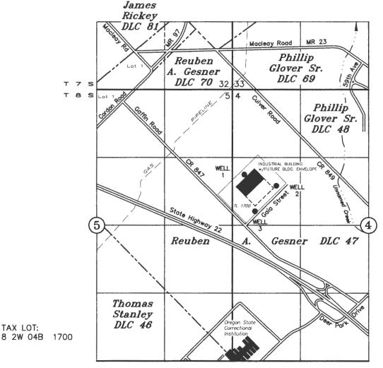
WELL 1: 2830' S & 945' E of the N'Iy NW COR REUBEN A. GESNER DLC No. 70 WELL 2: 3050' S & 1565' E of the N'Iy NW COR REUBEN A. GESNER DLC No. 70 WELL 3: 3550' S & 1150' E of the N'Iy NW COR REUBEN A. GESNER DLC No. 70
