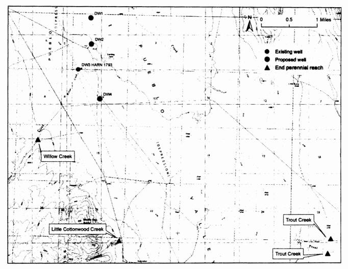
The nearest perennial stream reach to the existing and proposed wells is Willow Creek. The distance from the well to perennial reach, and the elevation difference between the well and the end of the perennial reach are given in the table below.
