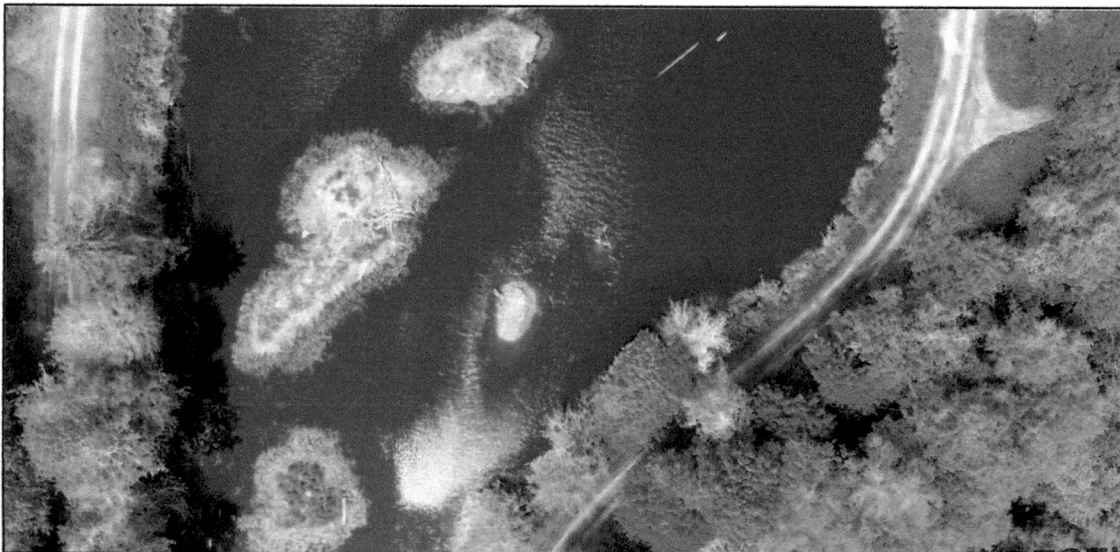
Figure 4-3. Islands in the pond would be lowered and flattened to support wetland vegetation and an increased varial zone as the pond water surface fluctuates.
