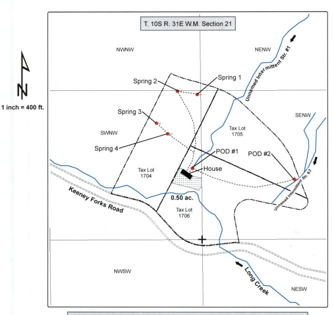
Spring 1: 1256' N, 29' W, Spring 2: 1275' N, 203' W, Spring 3: 1004' N, 381' W Spring 4: 911' N, 292' W Within the SWNW of Section 21, T. 10S R. 31E W.M. All measurements from the SE corner of the SWNW of Section 21, T. 10S R. 31E W.M.
