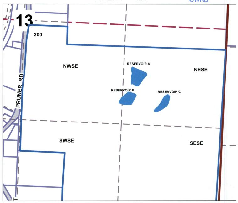
Reservoir A is 615 ft South and 1540 ft East from the Center of Section 13
