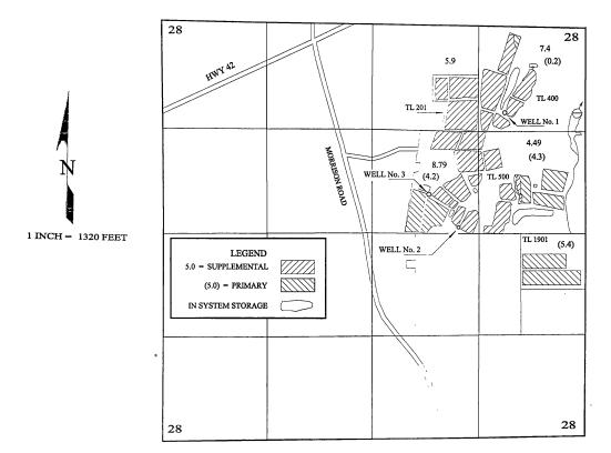
WELL No. 1 IS LOCATED 1490 FEET NORTH AND 990 FEET WEST, BEING WITHIN THE NE½NE½; AND WELL No. 2 IS LOCATED 80 FEET NORTH AND 1570 FEET WEST, BEING WITHIN THE SW½NE½; AND WELL No. 3 IS LOCATED 490 FEET NORTH AND 1940 FEET WEST, BEING WITHIN THE SW½NE½; ALL FROM THE EAST QUARTER CORNER OF SECTION 28 AND WITHIN SECTION 28, TOWNSHIP 28 SOUTH, RANGE 14 WEST, W.M.; COOS COUNTY.
