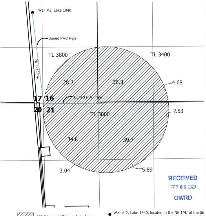
160.7 Acres of Primary Irrigation From Well #2, As Shown  Well # 2, Lake 1840, located in the NE 1/4/ of the SE 1/4 Section 17 & 2145' North and 245' West from the SE corner Section 17.
