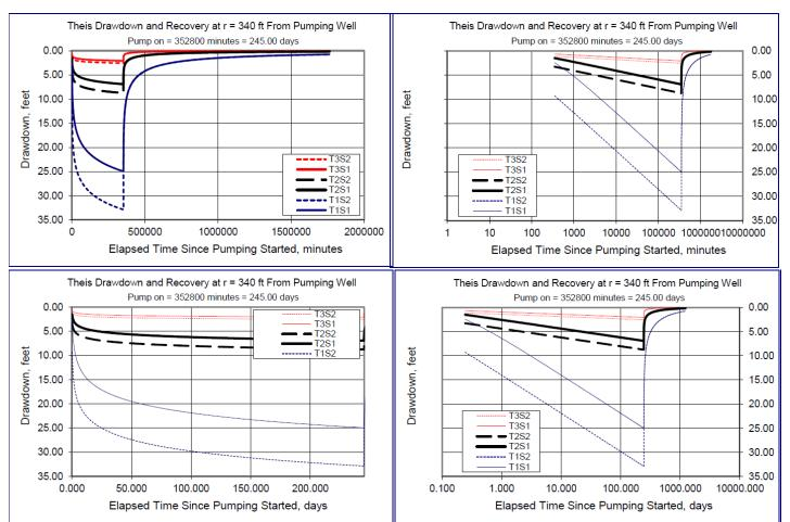
Transmissivity values from nearby pumping tests
