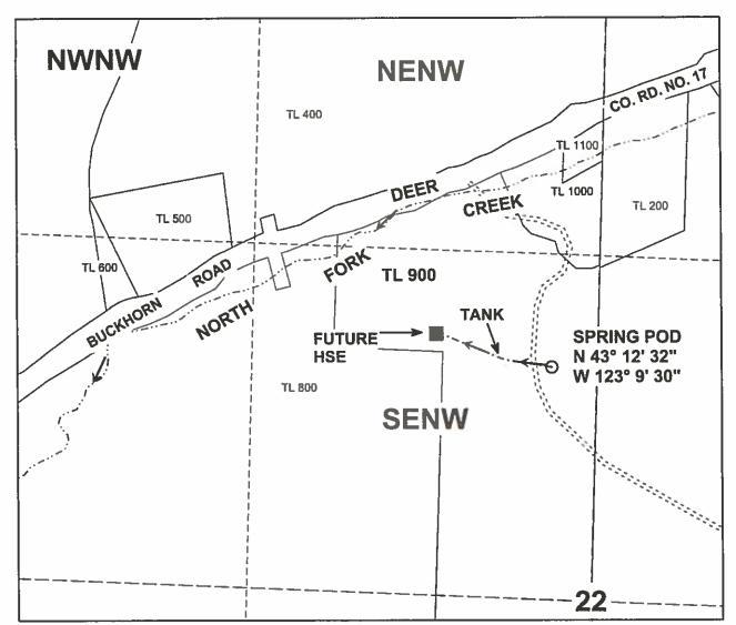
PROPOSED POD IS LOCATED 896 FEET NORTH AND 165 FEET WEST FROM THE C1/4 CORNER OF SECTION 22.
