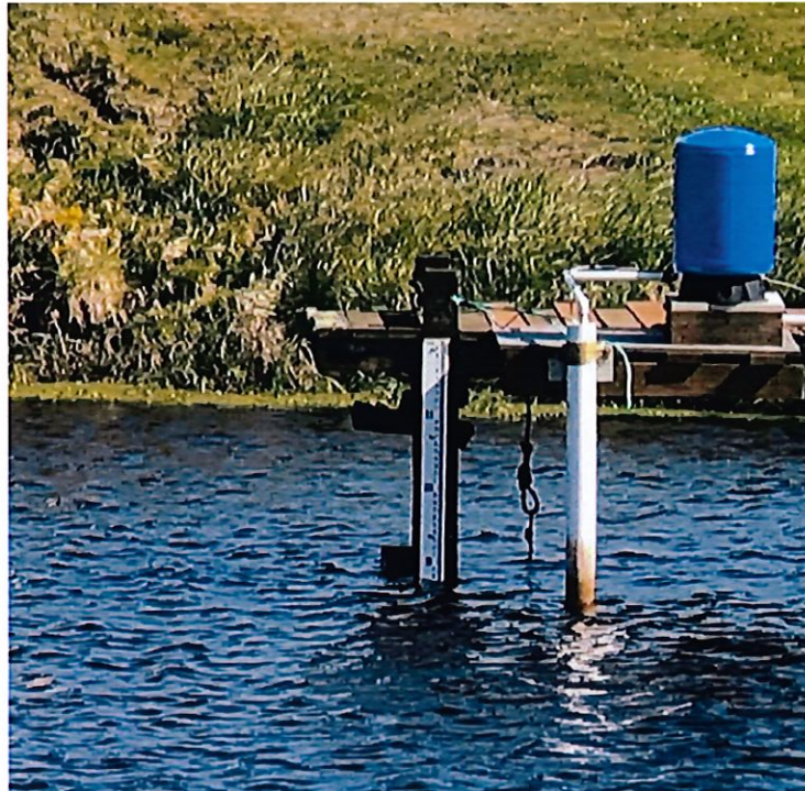
Staff gage at the end of the walk way, rectangular flash board stand pipe visible to left of the staff gage.
