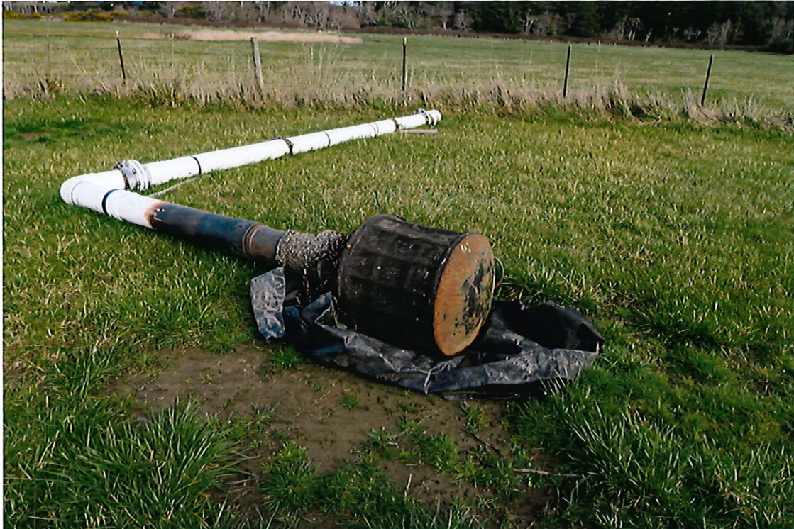
Active fish screen at the Two Mile Creek POD.
