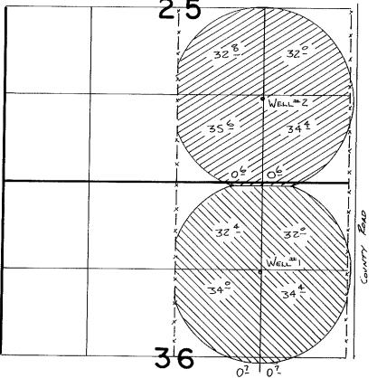
WELL#1 Loc: 1350'S : 1310'E } WELL#2 Loc: 1270'N, : 1300'E FROM N/4 COR SEC 36
