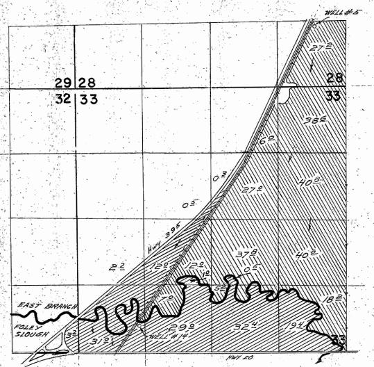
WELL #14 LOCATED 520 ft. N. E 1200 ft. E. FROM S.W. Cor. Sec. 33. WELL #5 LOCATED 100 ft. S. E. 620 ft. W. FROM N.E. Cor. SE/4 SE/4 Sec. 28.
