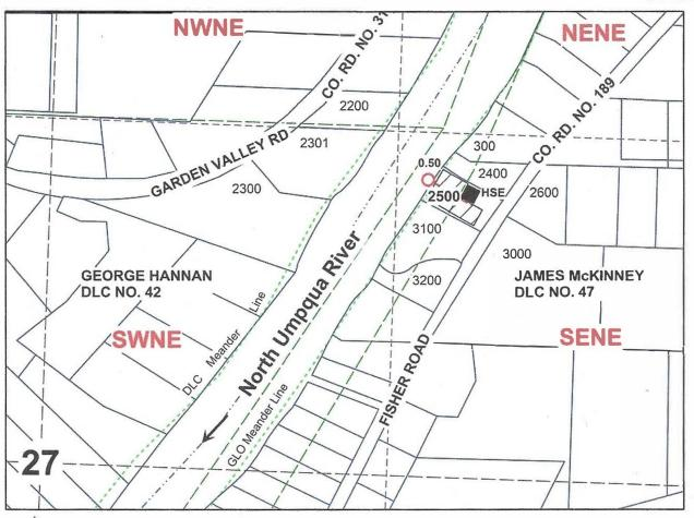
PROPOSED POD TO BE LOCATED 1109 FEET NORTH AND 1440 FEET EAST FROM THE CENTER CORNER, SECTION 27 AS PROJECTED IN DLC NO. 47.
