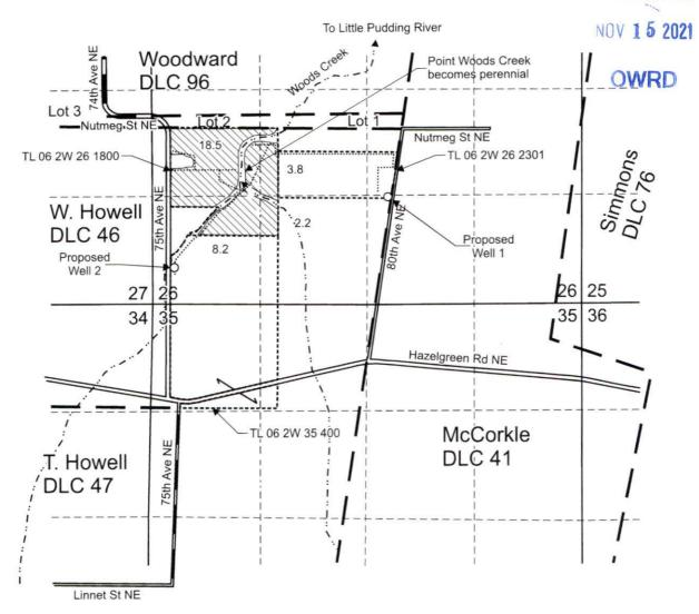
Proposed Well 1 is located 1,310 feet north and 2,380 feet west from the SE corner, Section 26. Proposed Well 2 is located 445 feet north and 265 feet east from the SW corner, Section 26.
