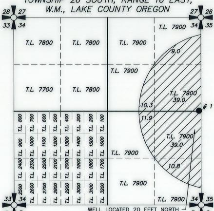
WELL LOCATED 20 FEET NORTH AND 60 FEET WEST OF THE EAST 1/4 CORNER OF SECTION 34. FLOWMETER LOCATED 5' SOUTHEASTERLY FROM WELL
