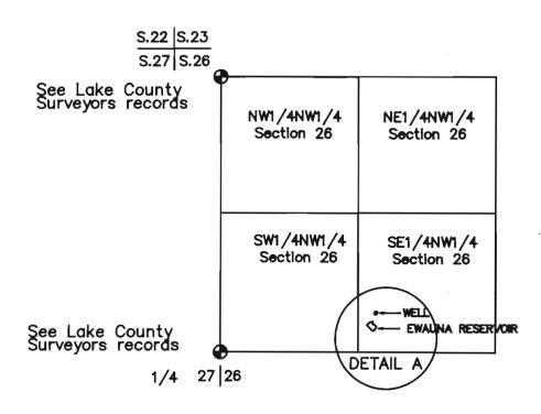
The center of Ewauna Reservoir is located S.31°21'52"E., 2750.46 ft., from the NW section corner of section 26. The measurement is from GPS survey by Peter A. Olson in 1999. The bearings are based on GLO record bearing of N.0°04"W., for the north half of the west line of section 26, as shown on the official survey approved June 1, 1935. The water stored in this reservoir is to be used for fire suppression activities, maintenance of Forest Service roads and stock watering.
