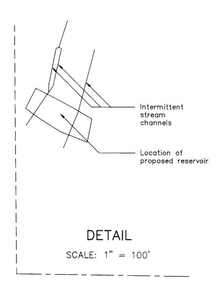
The center of the proposed reservoir is located S. 32°10'28" E., 2,710.06 feet from the northwest corner of section 26, T. 37 S., R. 16 E., W.M. This bearing is based on the G.L.O. record bearing of N. 0'04' W. for the north half of the west line of section 26 as shown on the official survey approved June 1, 1935. The water stored in this reservoir is to be used for fire suppression activities, maintenance of Forest Service roads, and stock watering.
