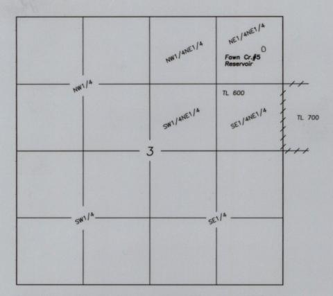
There is no outlet, the dam is located  $630^{\circ}$  South &  $350^{\circ}$  West of the NE corner of Section 3.
