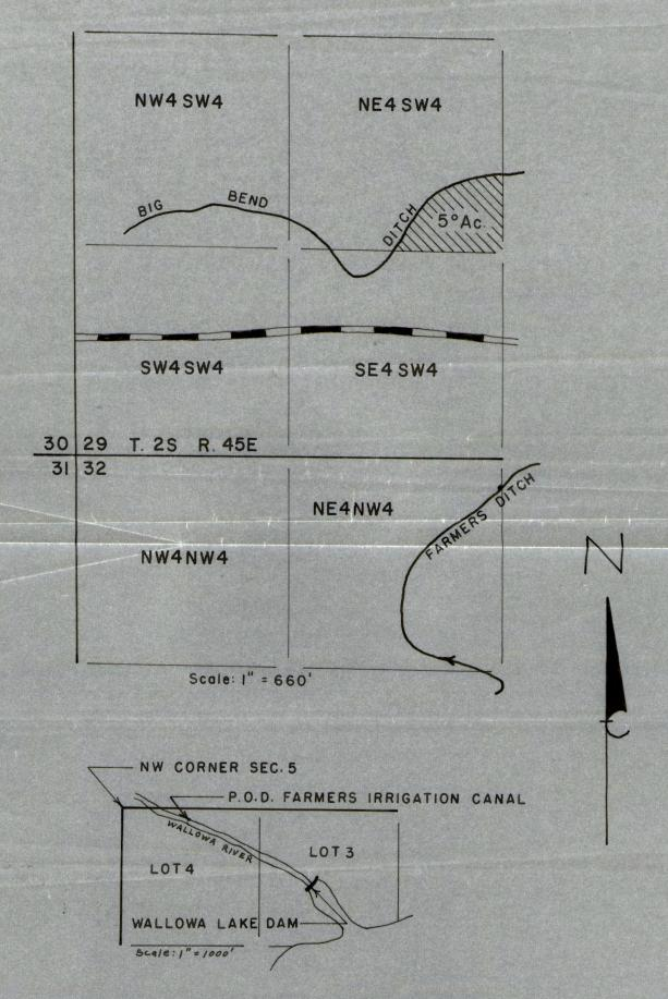
P.O.D. - S77°20'E a distance of 624 feet from the NW Corner of Sec. 5, T. 3S, R. 45E.
