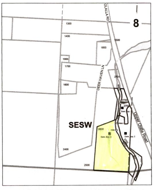
Point of Diversion 1 is 1410 ft. South and 220' West from the center of Section 8 Point of Diversion 2 is 1760 ft. South and 250' West from the center of Section 8 Point of Diversion 3 is 1880 ft. South and 240' West from the center of Section 8
