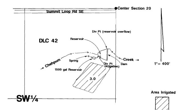
Div Pt (reservoir) located 590'S & 130'W from center of Section 20. Dam located 680'S & 120'W from center of Section 20. Ov Pt (irrigation) located 700'S & 230'W from center of Section 20.
