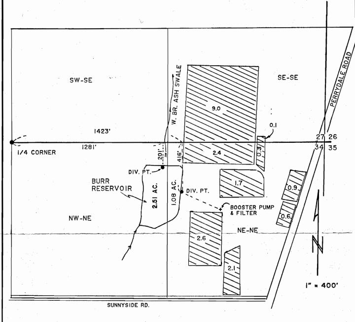
THE DIVERSION POINT FOR THE RESERVOIR IS 1281 FT. EAST AND 201 FT. SOUTH OF THE SOUTH 1/4 CORNER OF SECTION 27. THE DIVERSION POINT FOR THE IRRIGATION IS 1423 FT. EAST AND 416 FT. SOUTH FROM SAID 1/4 CORNER.
