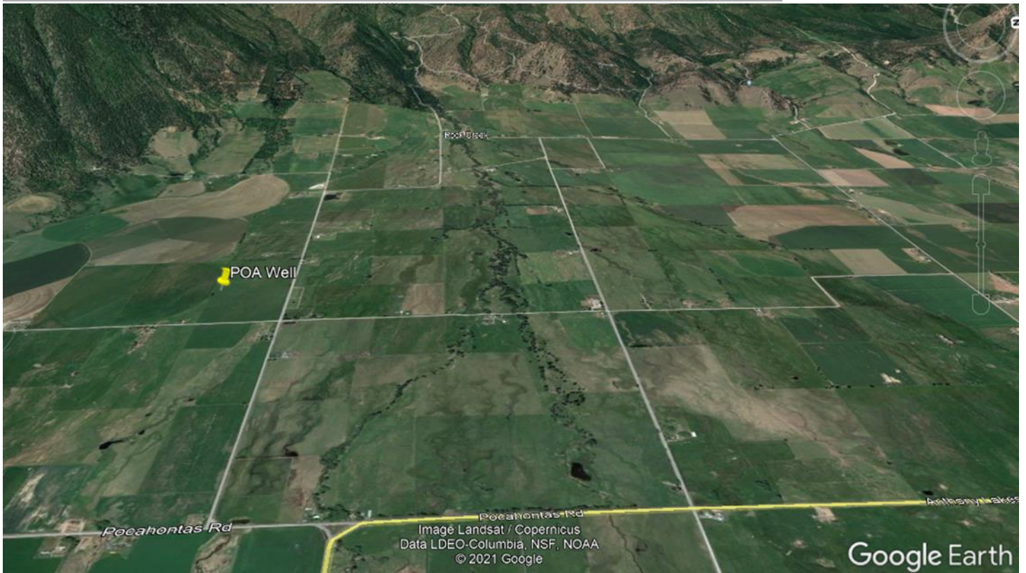
View of the Rock Creek alluvial fan looking west along the axis. The depositional regime of alluvial fans results in a heterogeneous sequence with much higher transmissivity parallel to the axis of the fan.
