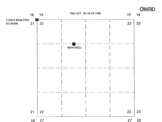
NEW WELL LOCATED IN THE NE1/4NW1/4 OF SECTION 22 AND LOCATED 1997 FEET EAST AND 1327 FEET SOUTH FROM THE NW CORNER OF SECTION 22, T39S, R19E, WM, LAKE COUNTY, OREGON
