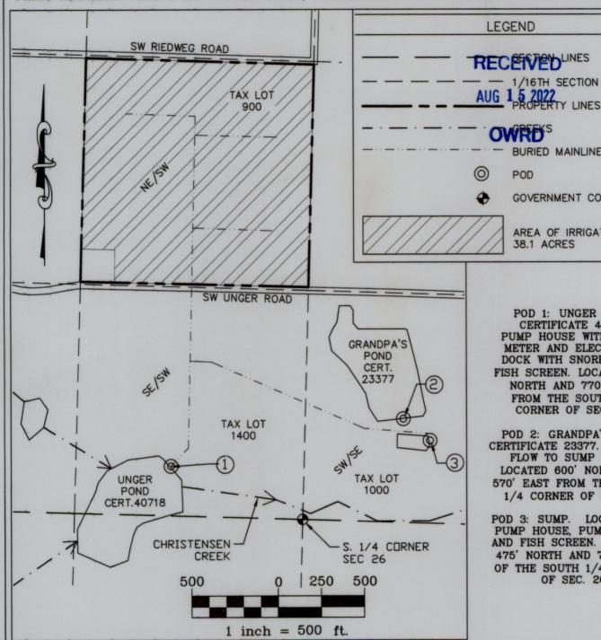
POD 1: UNGER POND, CERTIFICATE 40718. PUMP HOUSE WITH PUMP, METER AND ELECTRICAL. DOCK WITH SNORKLE AND FISH SCREEN. LOCATED 285' NORTH AND 770' WEST FROM THE SOUTH 1/4 CORNER OF SEC. 26.
