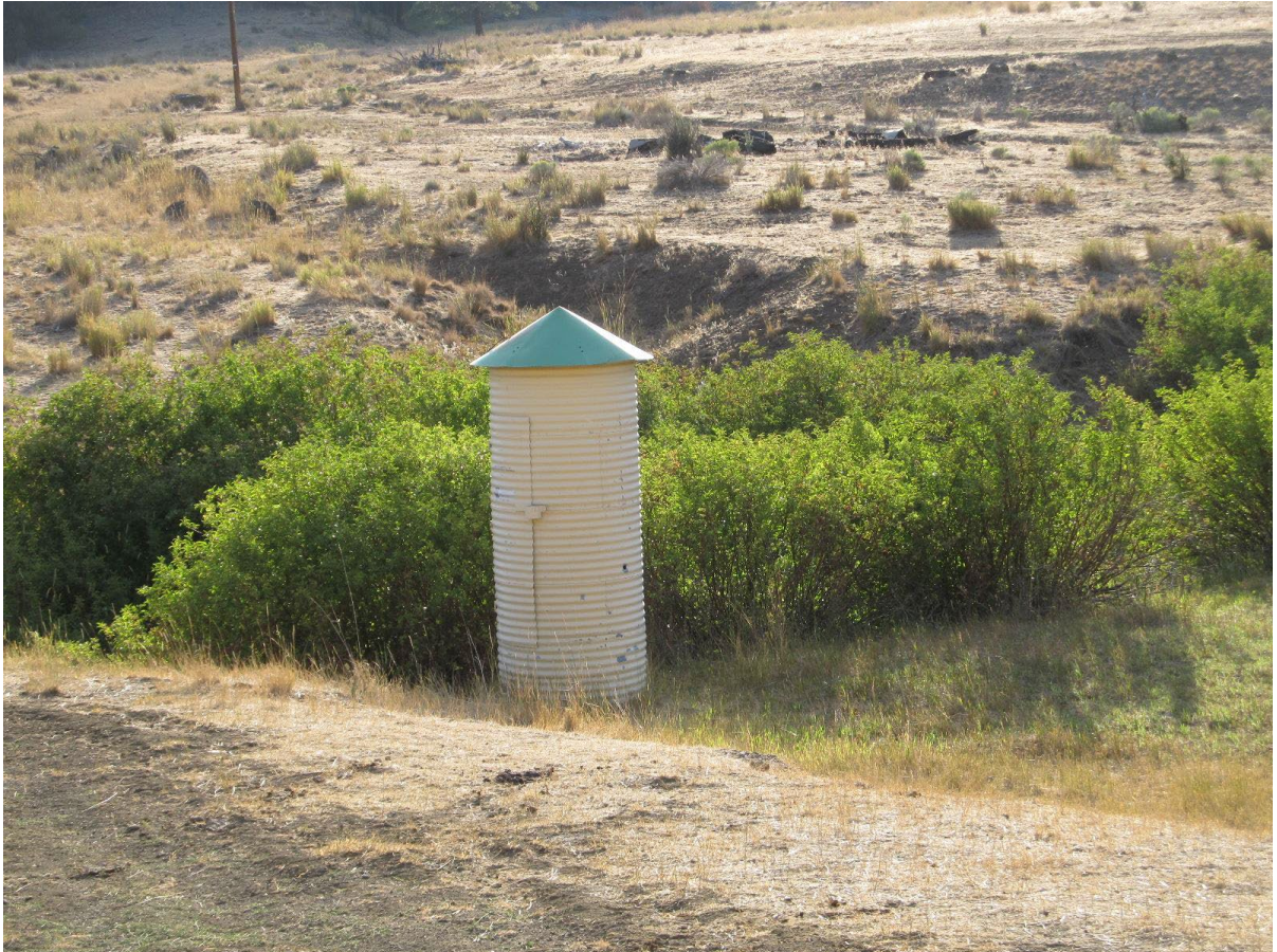
A stream gauge on the South Fork John Day River (Jeffrey Kee photo credit)
