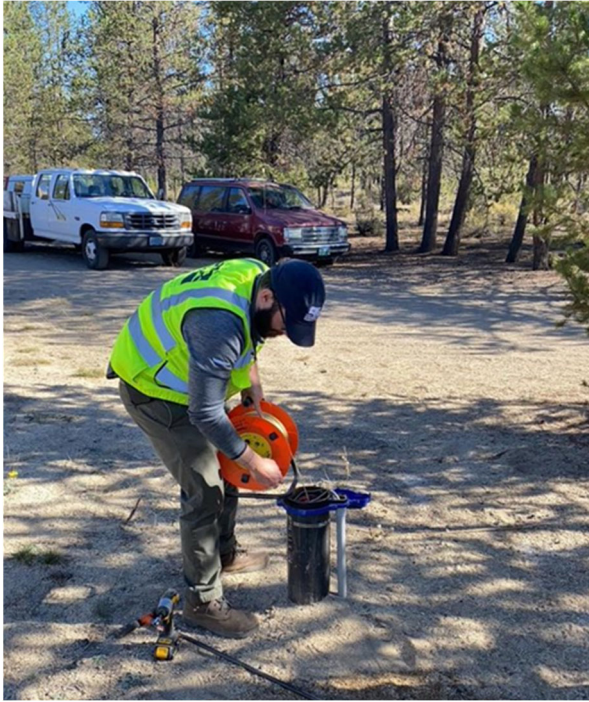
Inspector taking a static water level measurement
