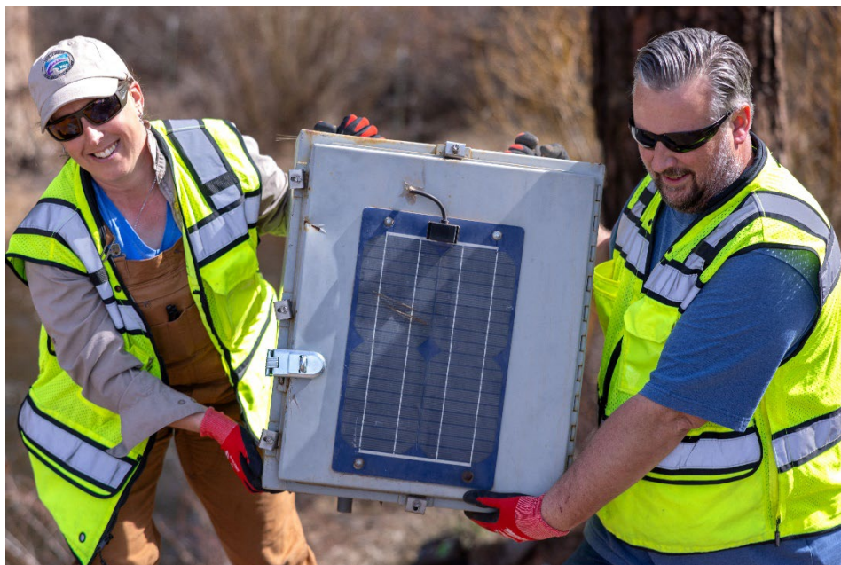
Watermasters Terra Kemper and Matt Anderson removing a defective gage station.
