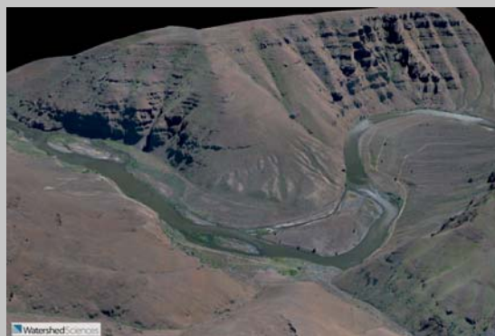
LiDAR-derived terrain model John Day, Oregon. Data collected for the Oregon Parks and Recreation Department
