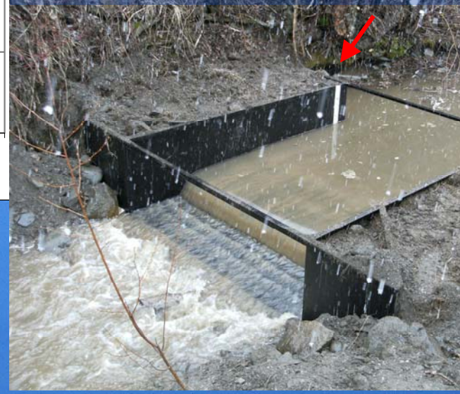
Ramp flume with staff gage
