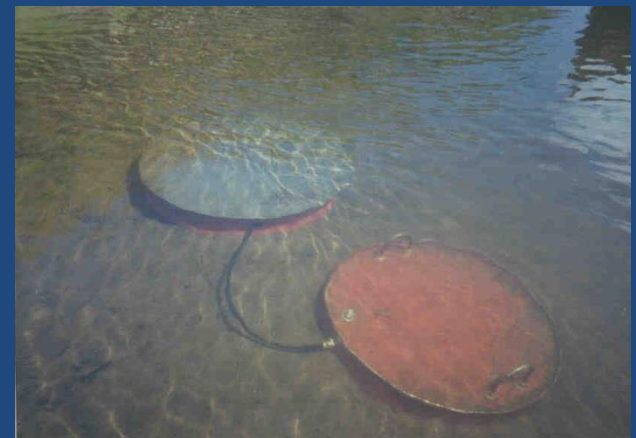
Seepage meters recording groundwater discharge to the Pudding River in the Willamette basin
