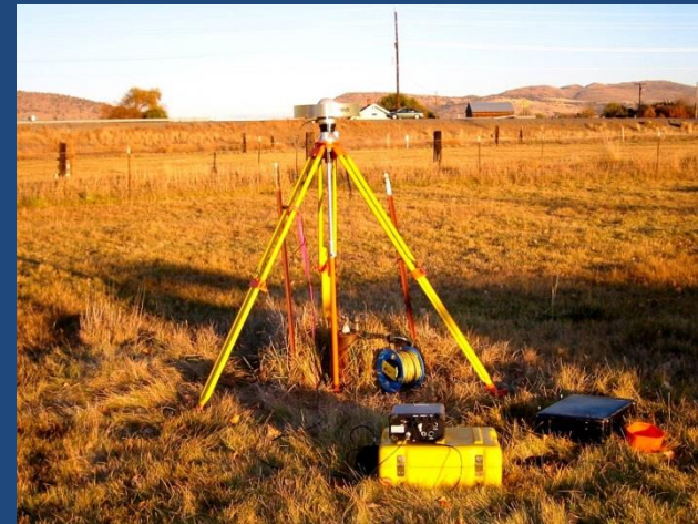
GPS leveling survey for wells in the Klamath basin
