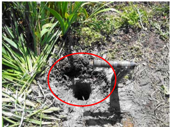
Figure 9. Abandonment with Slumping Seal.
