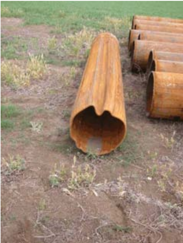
Left - Casing damaged during construction.
