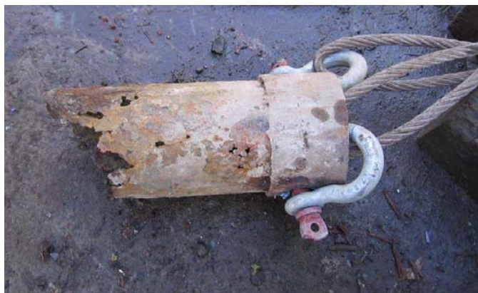
This piece of rusty casing is from a well abandonment. The casing was so corroded and pitted that it pulled apart during abandonment work.
