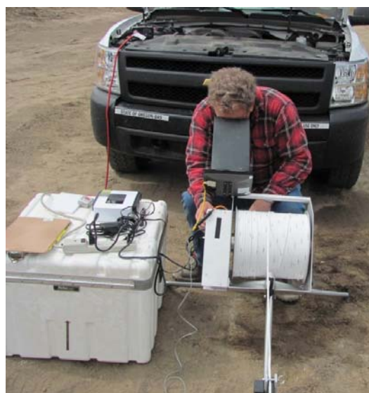
East Region Well Inspector viewing inside a well using a video camera.
