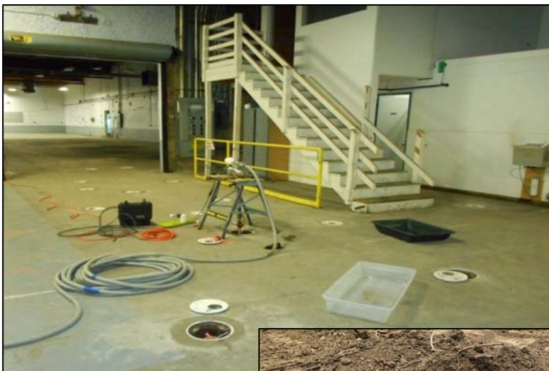
An injection system connected to a single remediation well.
