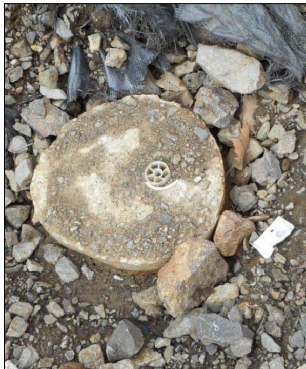
Damaged Continuous Multichannel Tubing (CMT) monitoring well that was later decommissioned by over-drilling.
