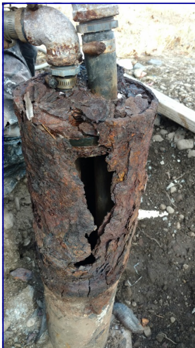
Well casing damaged by water treatment chemicals.
