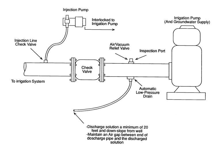
Backflow prevention device using check valve with vacuum relief and low pressure drain.
