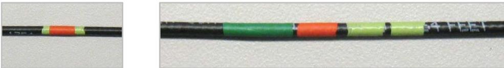
The coaxial water level meter has a thin line (like a speaker wire) marked in five-foot increments. Determining how much line you have in the well requires counting the color-coded markers using a pattern similar to adding with Roman numerals.
