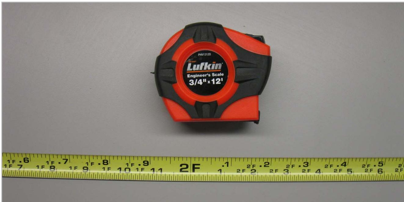
Co-axial e-tape measurements require the additional use of an engineer's tape measure to obtain measurements to the nearest 1/100<sup>th</sup> foot. The engineer's tape measure is marked in feet, 1/10<sup>th</sup> foot, 1/100<sup>th</sup> foot, and inches.
