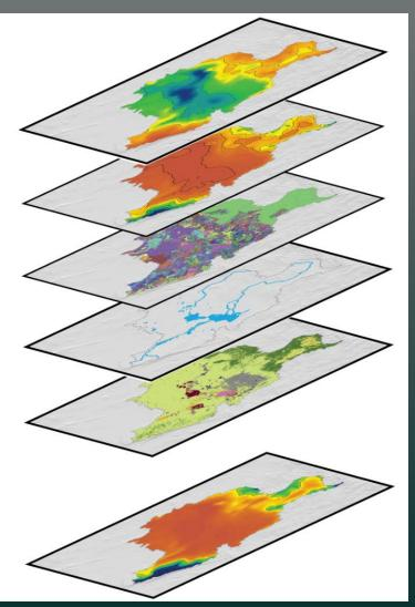
Precipitation<sup>1</sup> Evapotranspiration Soils<sup>1</sup> Runoff Land use<sup>1</sup> **Upland recharge**
