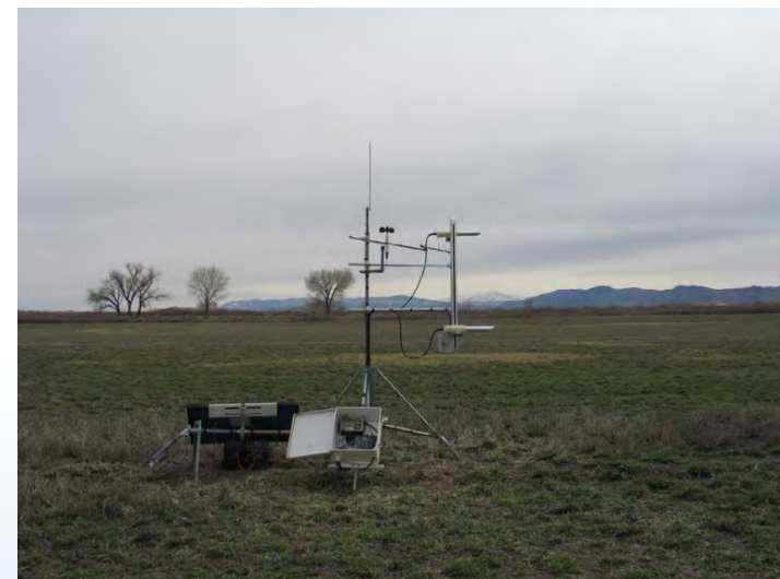
Bowen Ratio ET station in a flood irrigated alfalfa field in Walker River Valley, NV
