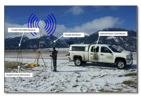
A Trimble R10 base station antenna located over a known reference point. Corrected GPS position and elevation information is transmitted either by Internal Radio or by a Trimmark III base radio to the R10 GPS rover unit.
