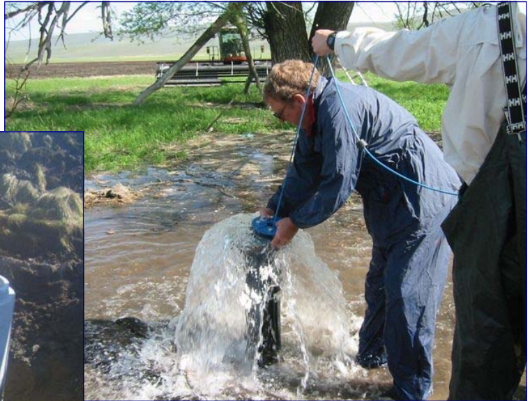
Preparing to video a flowing artesian well.
