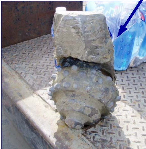
The drill bit that was retrieved from the borehole, using the homemade tool.
