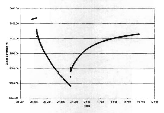
Figure B-3 Reservoir Well Hydrograph Constant Rate Aquifer Test Baker City ASR Reservoir Well Study
